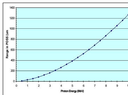
**Figure 4:** Proton range-energy curve in POSS with 1.2 g/cm<sup>3</sup> density
