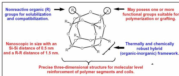
**Figure 1:** Anatomy of a POSS<sup>®</sup> nanostructured<sup>®</sup> chemical
