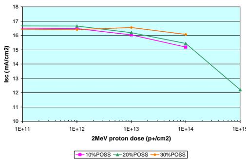
Figure 13: Calculated  $I_{sc}$  variation with 2 MeV proton dose for MA8000-coated samples
