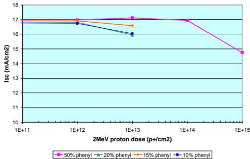
Figure 12: Calculated  $I_{sc}$  variation with 2 MeV proton dose for PM1287-coated samples
