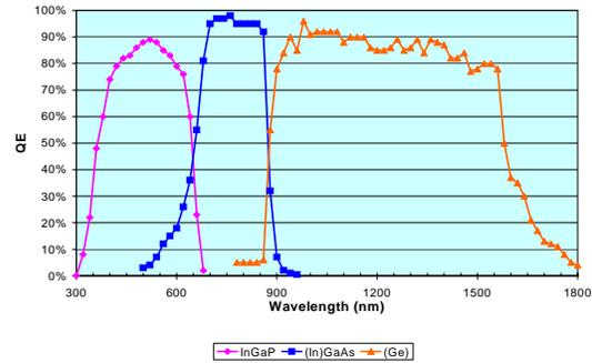
Figure 11: External quantum efficiency, ATJ cell
