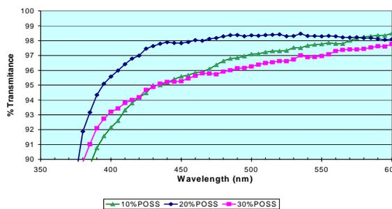
Figure 8: Spectral transmission curves of MA8000 with various POSS additions
