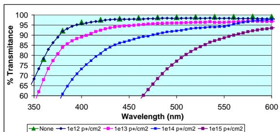
Figure 10: Spectral transmission curves of MA8000.2 with proton fluence
