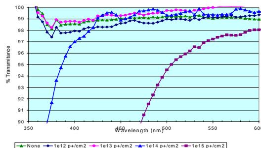
**Figure 5:** Spectral transmission curves of PM1287 with 50% phenyl
