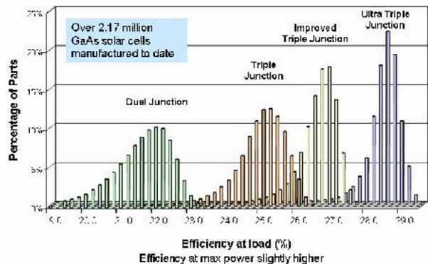
**Fig. 5** AM0 efficiency distributions of four generations of Spectrolab space solar cells.
