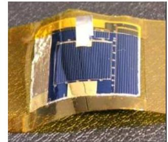
**Fig. 4** Picture of a 0.25 cm<sup>2</sup> IMM cell
