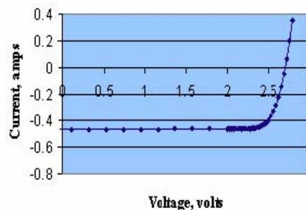
Fig. 1 Current-voltage curve for a 27.55 cm<sup>2</sup> BTJ solar cell.
