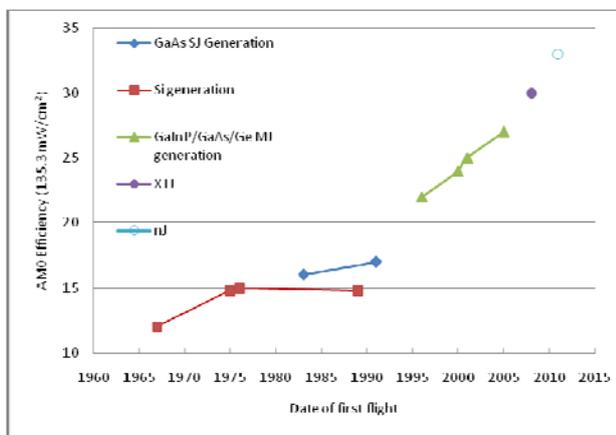
**Fig. 6** Solar cell efficiency with first launch to orbit
