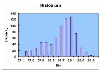
**Fig. 2** Histogram of AM0 efficiency of 700 BTJ cells
