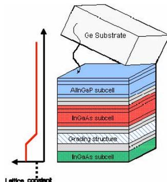
**Fig. 3** Schematic diagram of the IMM approach.
