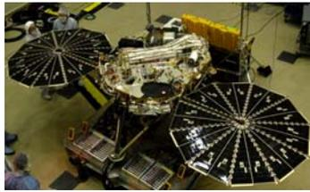
**Fig. 8** Ultraflex array on the Phoenix Mars lander
