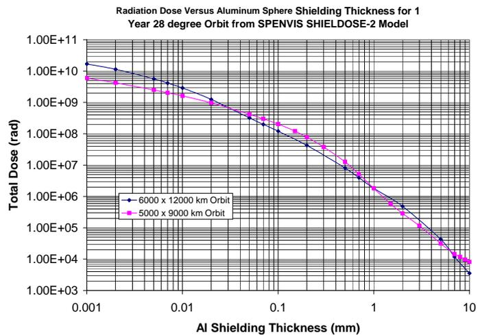
**Figure 6:** Total Dose versus shielding thickness
