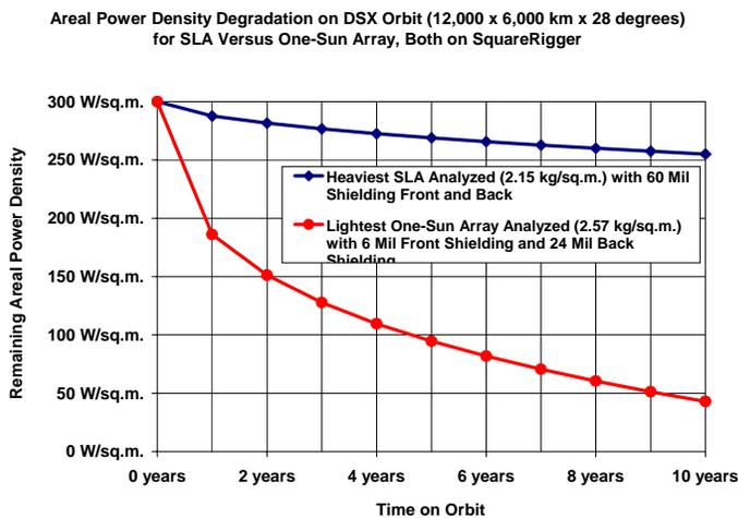
**Figure 5:** EOL Areal Power Density Comparison
