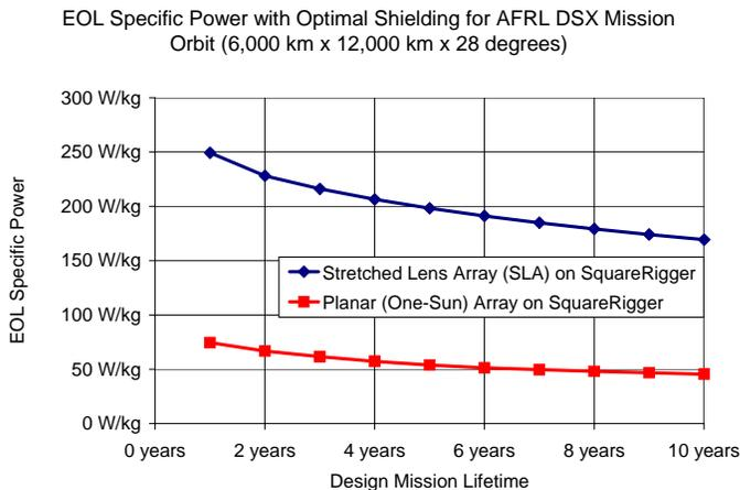
**Figure 4:** EOL Specific Power Comparison
