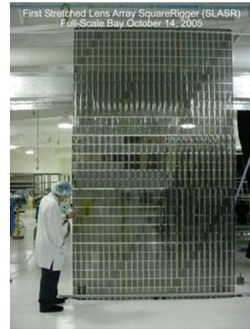
Figure 1: Full scale SLASR module
