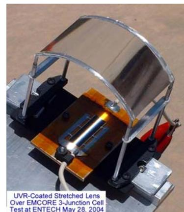
Figure 1: Sunlight testing of laser receiver assembly
