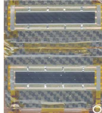
**Figure 9** - Stretched lens array module after testing
