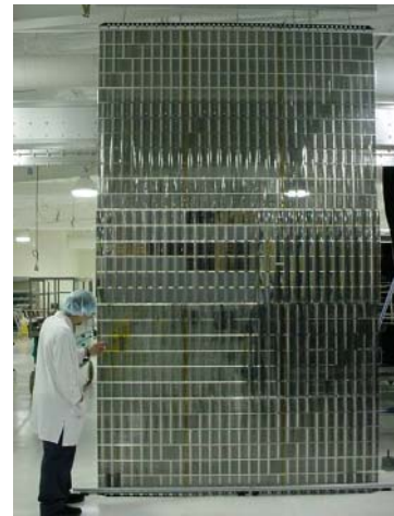
Figure 7. 3.75 kW Stretched lens array on a SquareRigger platform
