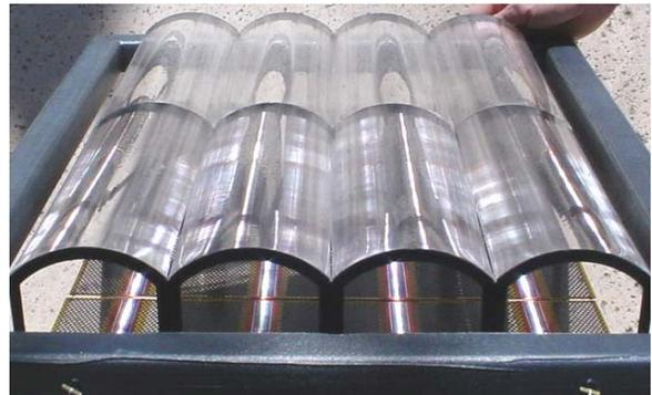
Fig. 1. Stretched lens array in sunlight
