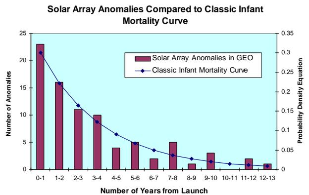
Fig. 3. Solar array anomalies compared to infant mortality curve
