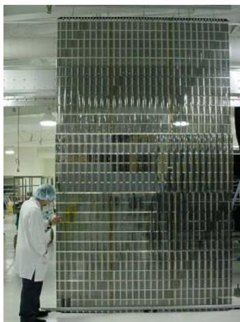
Fig. 6. 3.75 kW SLA on a SquareRigger platform
