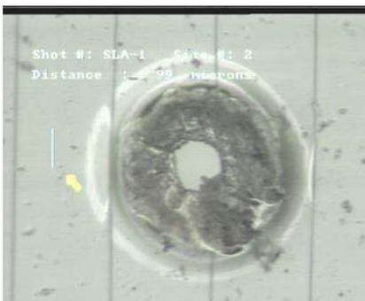
Fig. 9. Lens sample after hypervelocity shot
