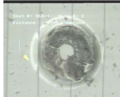
Fig. 5. Lens sample after hypervelocity shot
