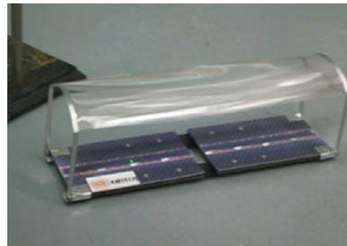
**Figure 11. Picture of wind distortion to lens with light remaining focused on cells**
