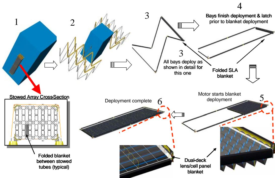
**Figure 3. Deployment of the SLASR**
