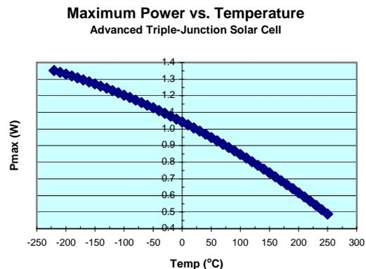
**Figure 8. Effect of temperature on the maximum power of an ATJ solar cell**
