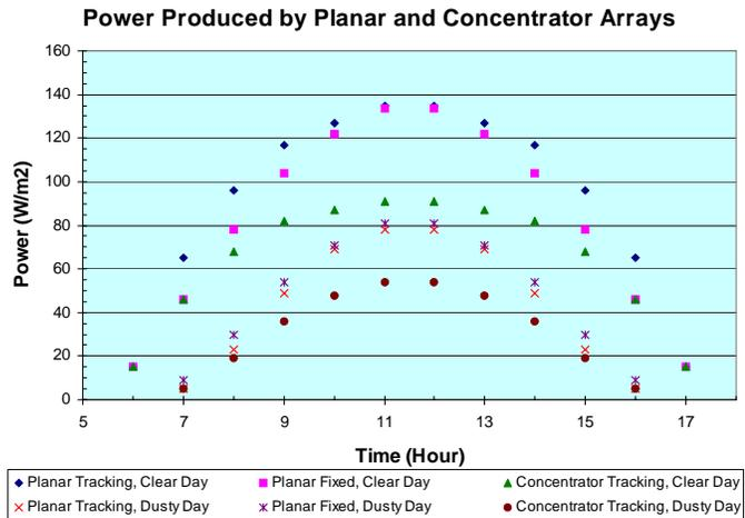
**Figure 6. Impact of Mars Atmosphere Conditions on Power Produced by Planar and Concentrator Arrays**
