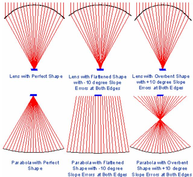
**Figure 10. Direct Ray-Trace Comparison of Shape Error Tolerance of ENTECH's Lens versus Reflective Concentrator**
