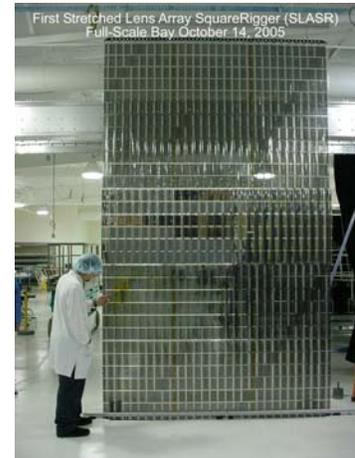
**Figure 2. Full scale SLASR module**
