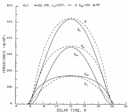
Figure 4. Global (top curve), direct beam (middle) and diffuse (bottom) insolation for a fixed horizontal surface (solid line) compared with a tracking surface (dashed line) for a relatively clear day ( $L_s=1530$ ) at Viking Lander site VL-1.<sup>8</sup>
