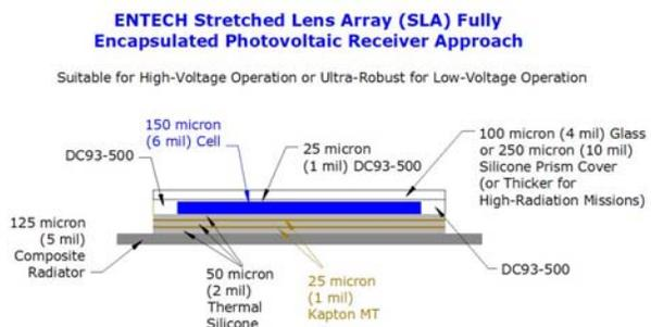
Figure 9. SLA receiver cross section
