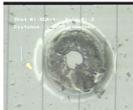
Figure 4: Lens sample after hypervelocity shot
