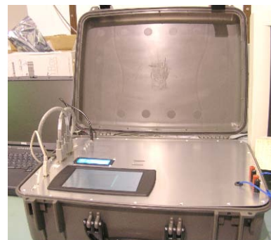
Fig. 10. Packaged DAS components with touch-screen GUI in a portable case.
