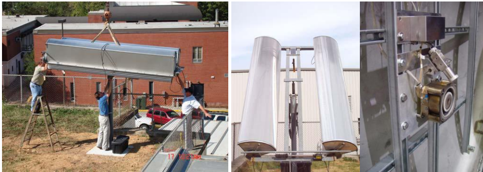
Fig. 4. (a),(b) Entech Solar SunLine installed at Auburn Univ. (c) T-100 Hall Thruster and cathode
